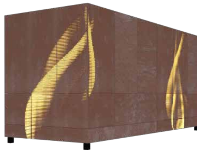
Container - ytterside klaffer - perforerte Corten plater
